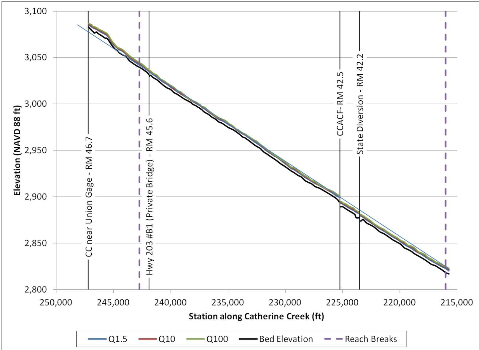
Figure 31. Computed water surface elevation for reach four on Catherine Creek.
