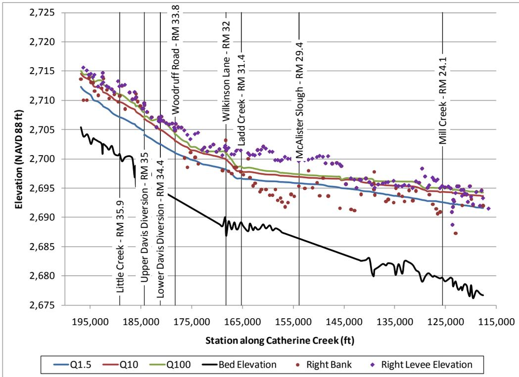
Figure 46. Reach 2 water surface profiles compared with levee and bank heights along the right bank.
