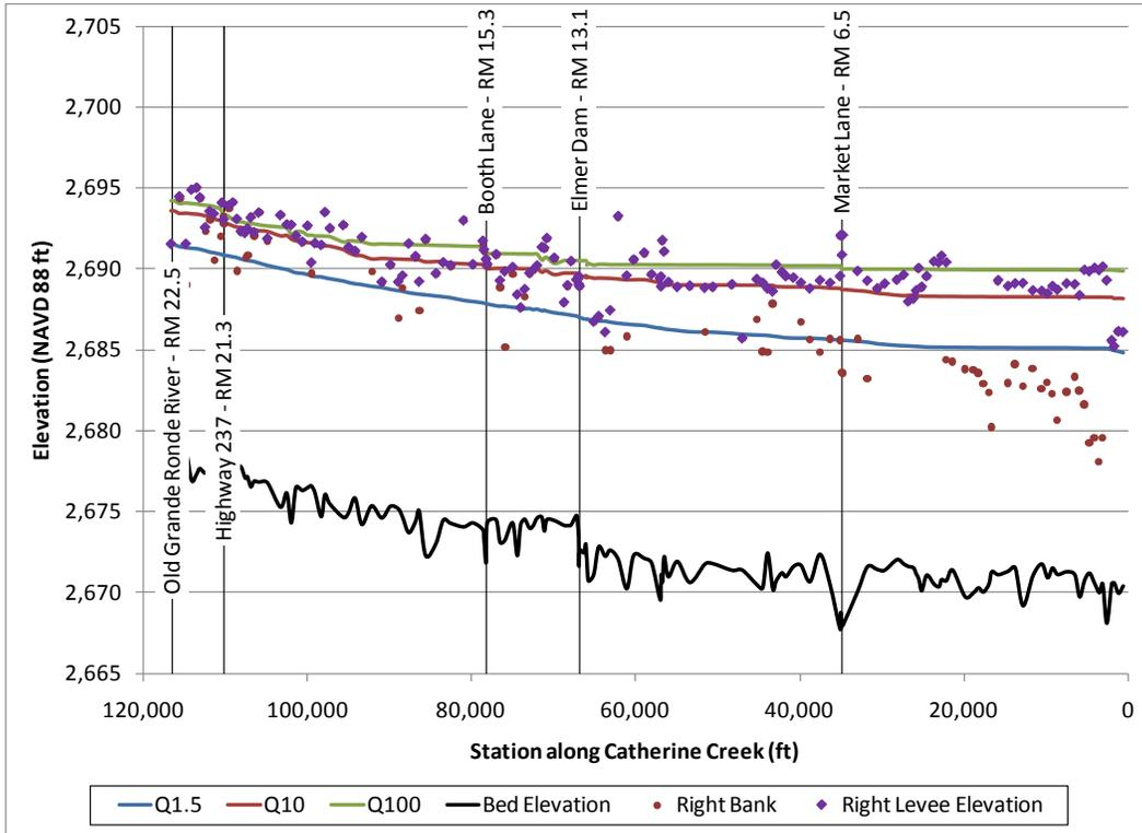
Figure 44. Reach 1 water surface profiles compared with levee and bank heights along the right bank.
