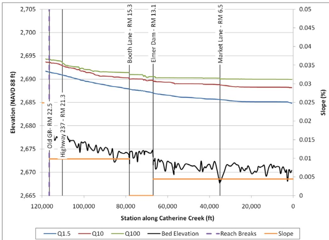
Figure 28. Computed water surface elevation for reach one on Catherine Creek.
