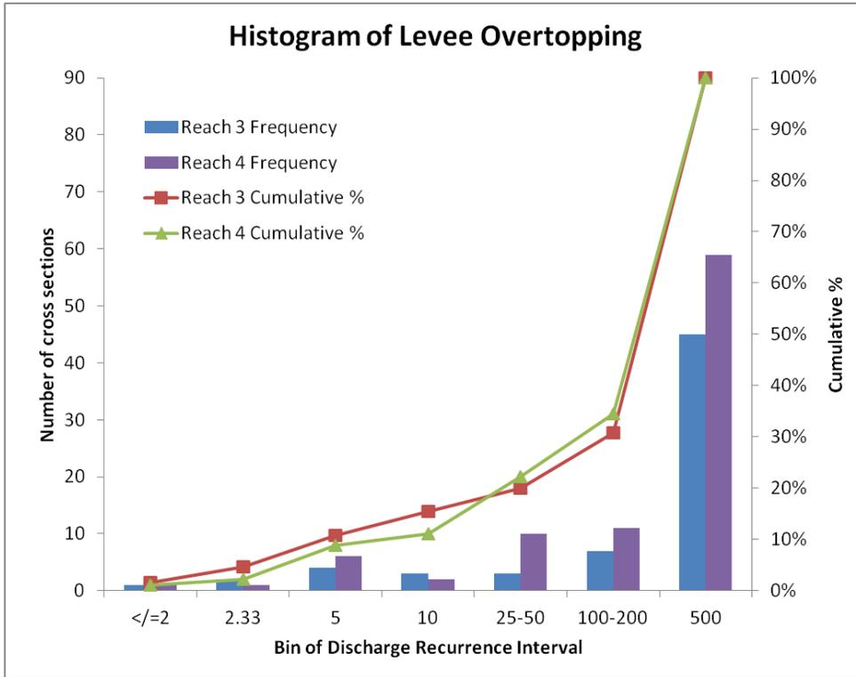
Figure 42. Distribution of cross sections overtopping levees at specific recurrence interval discharges within Reaches 3 and 4.
