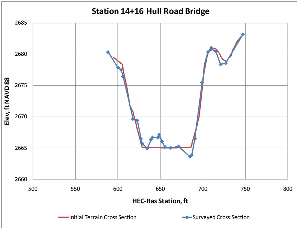
Figure 5. Example of channel cross section near bridge that was modified to include AP survey data.
