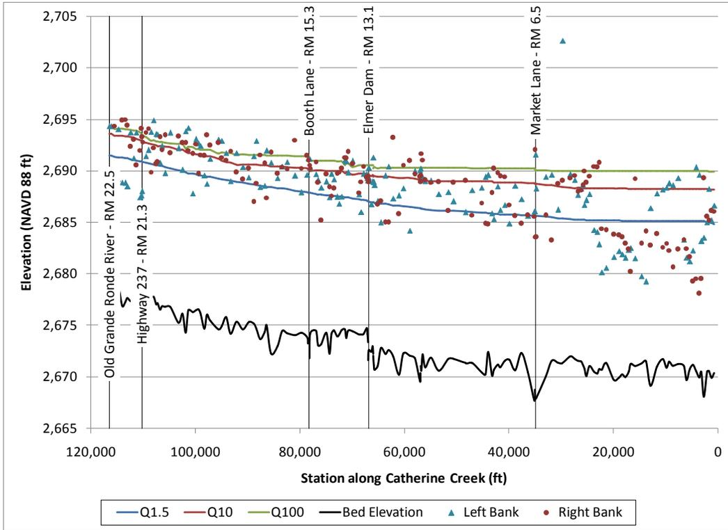
Figure 32. Comparison of bank elevations with flood discharges for Reach 1 of Catherine Creek.
