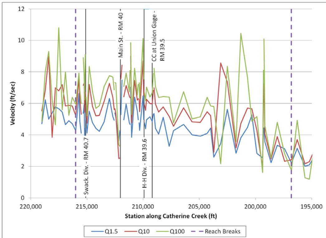
Figure 54. Computed cross-sectional average channel velocity for Reach 3 on Catherine Creek.
