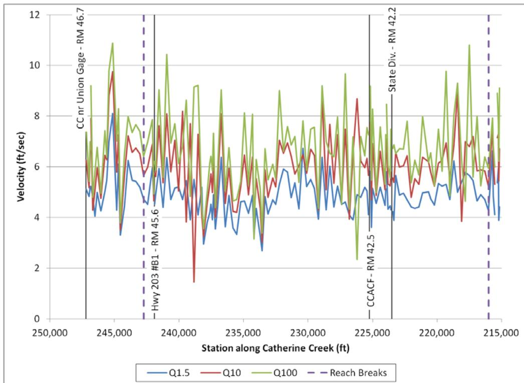
Figure 55. Computed cross-section average in-channel velocity for Reach 4 on Catherine Creek.
