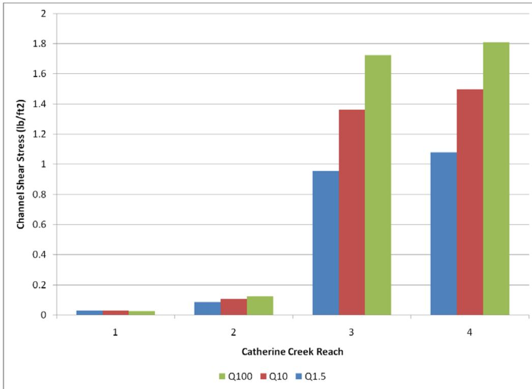
Figure 56. Reach averaged channel shear stress on Catherine Creek.
