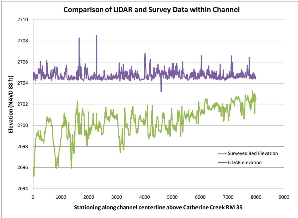
Figure 2. Comparison of LiDAR data within the channel and surveyed bed elevations.
