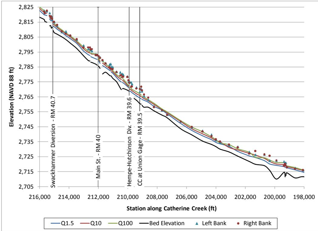
Figure 34. Comparison of bank elevations with flood discharges for Reach 3 of Catherine Creek.
