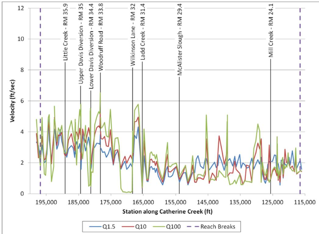
Figure 53. Computed cross-section average in-channel velocity for Reach 2 on Catherine Creek.
