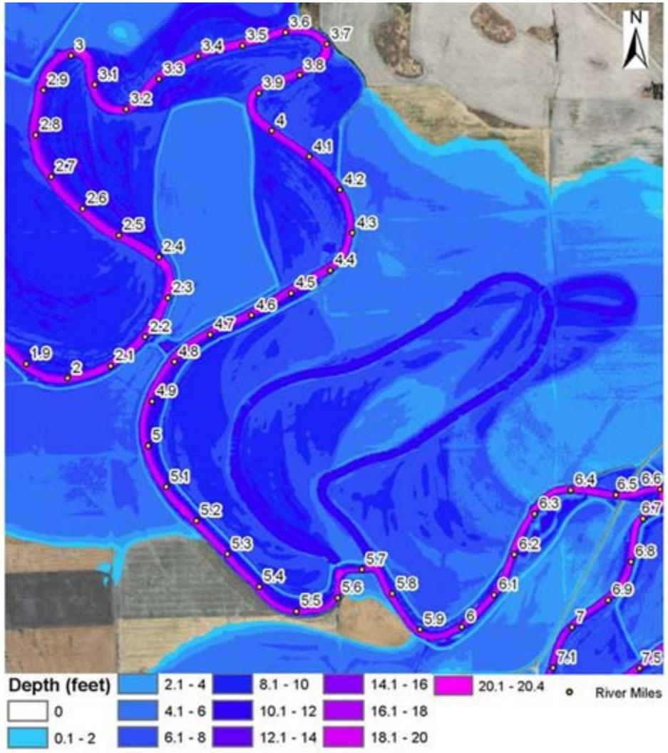
Figure 48. Potential flooding depths within the bounds of the modeled cross sections for the 100-year discharge in a portion of Catherine Creek Reach 1.
