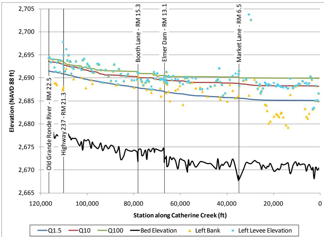
Figure 43. Reach 1 water surface profiles compared with levee and bank heights along the left bank.
