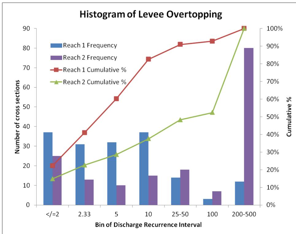
Figure 41. Distribution of the number of cross sections overtopping levees at specific recurrence interval discharges within Reaches 1 and 2.
