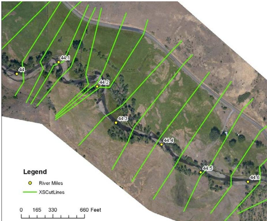
Figure 3. Example portion of upper Catherine Creek with delineated cross sections.
