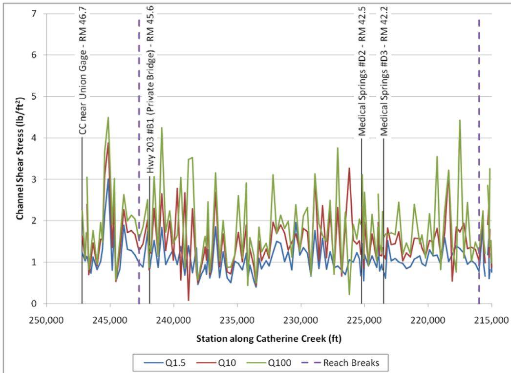
Figure 57. Channel shear stresses in Reach 4 on Catherine Creek.
