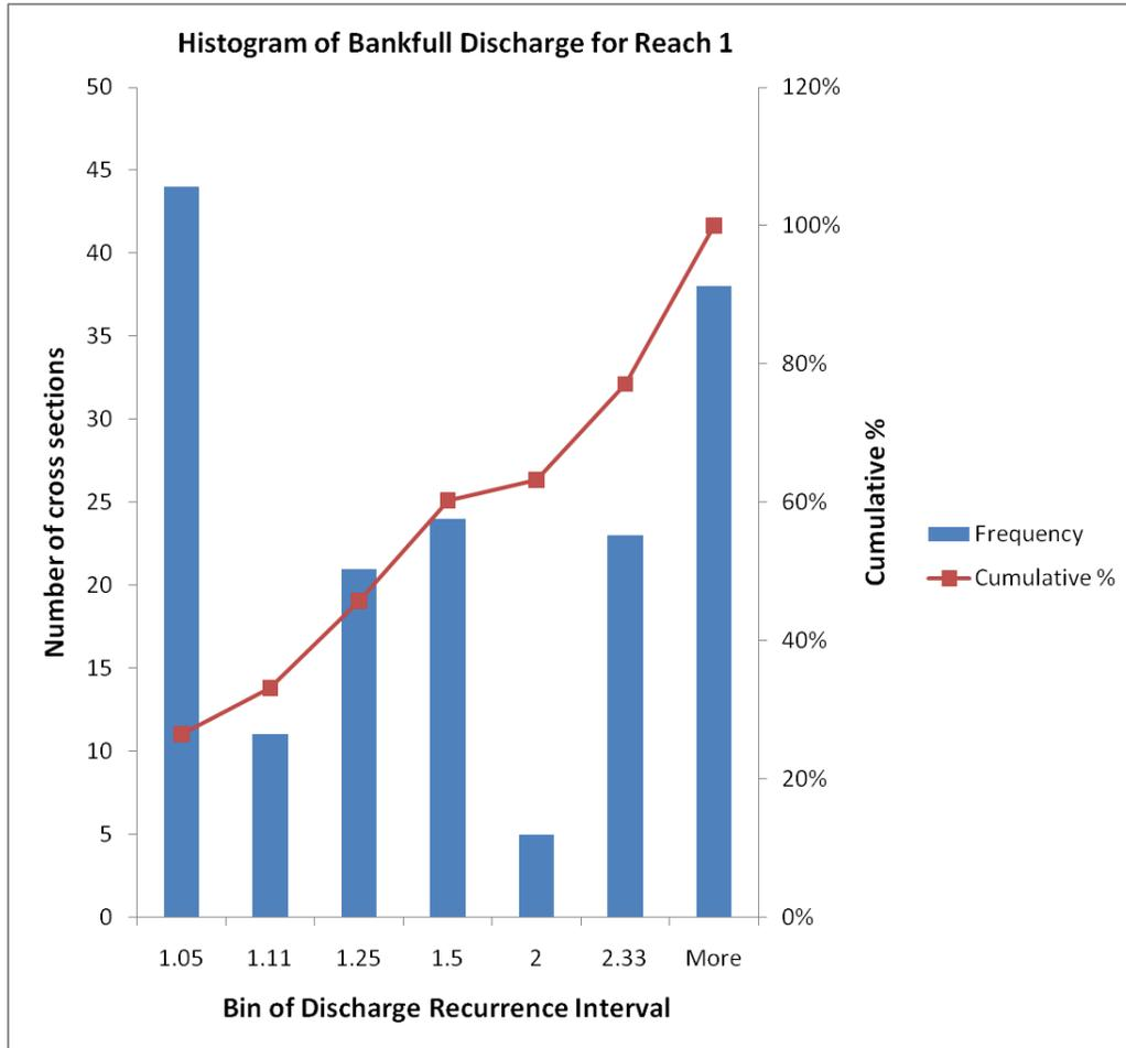
Figure 40. Plot of the distribution of bankfull discharges for cross sections in Reach 1.
