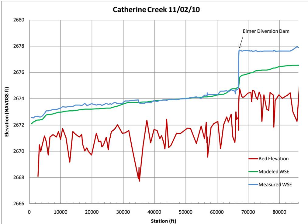
Figure 19. Measured versus modeled water surface elevations for Catherine Creek RM 0 to RM 16.3, measured on 11/02/2010.
