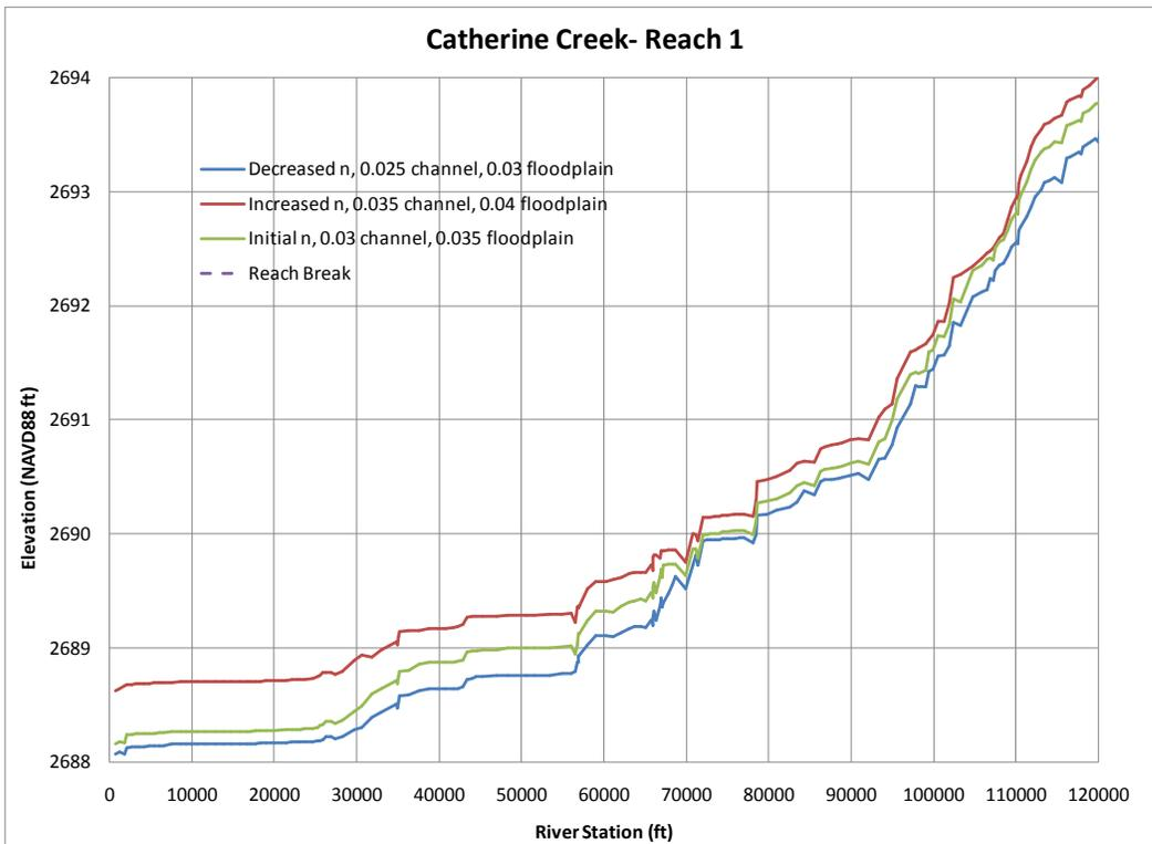
Figure 24. Sensitivity to Manning's n at a 10- year discharge for Reach 1 of Catherine Creek.
