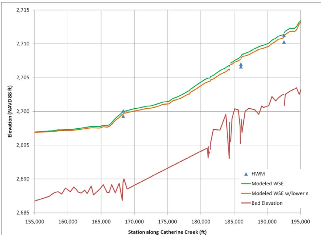
Figure 15. Modeled water surface elevations versus measured high water marks for Catherine Creek (RM 29.6 to 36.5).
