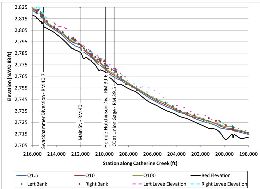
Figure 47. Reach 3 water surface profile compared with levee elevations.
