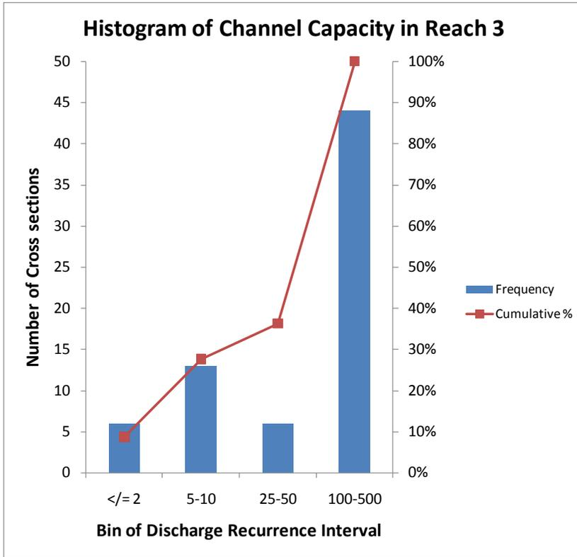
Figure 38. Distribution of channel capacity recurrence intervals for cross sections in Reach 3.
