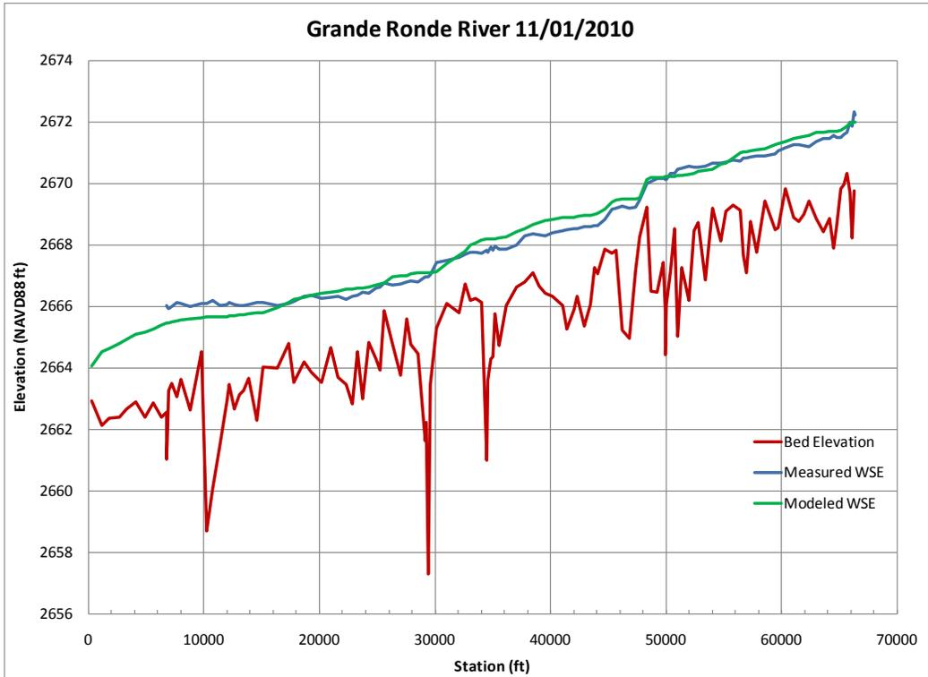
Figure 17. Measured versus modeled water surface elevations for Grande Ronde River downstream of State Ditch, measured on 11/01/2010.
