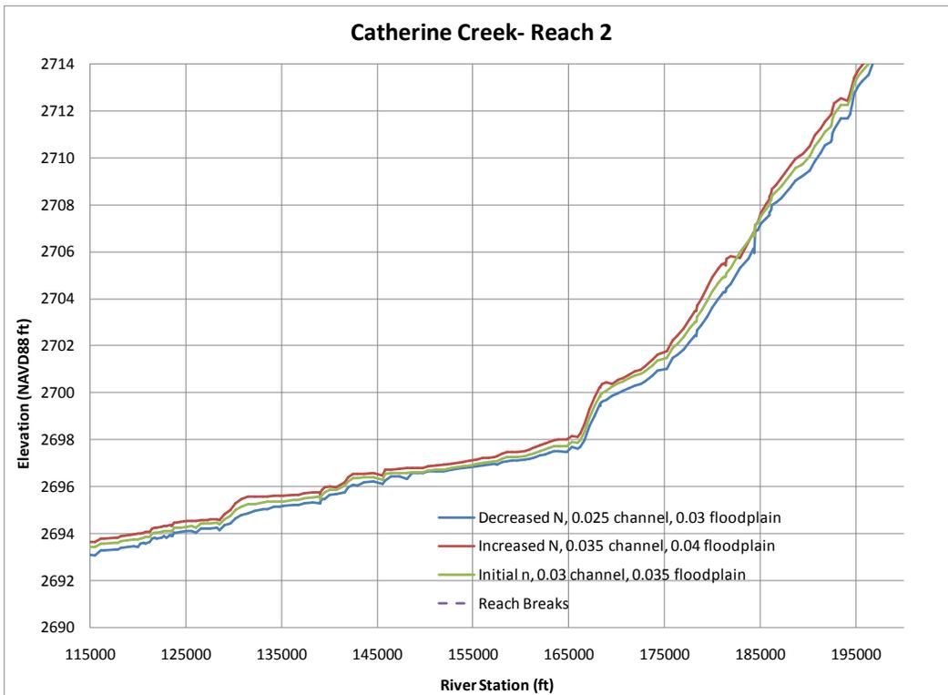
Figure 26. Sensitivity to Manning's n at a 10- year discharge for Reach 2 of Catherine Creek.
