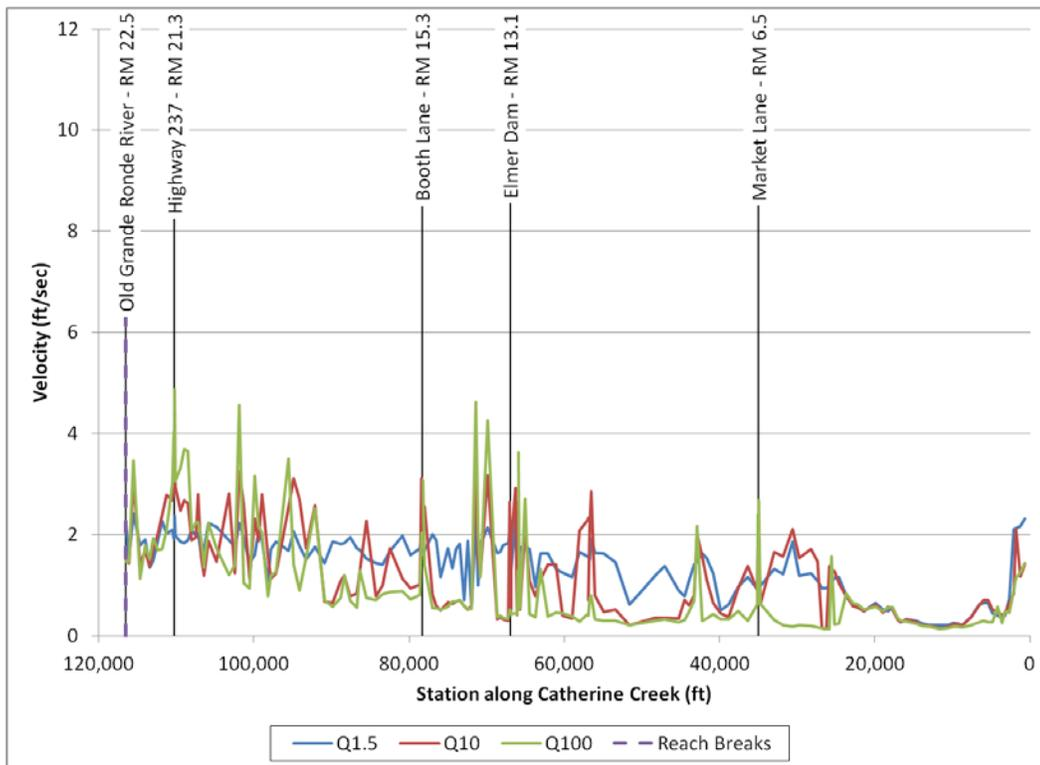
Figure 52. Computed cross-section average in-channel velocity for Reach 1 on Catherine Creek.
