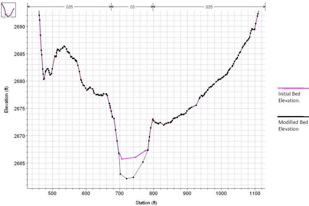
Figure 9. Example of channel bed modification to downstream-most 9 cross sections. Cross section shown is at station 1198.25.
