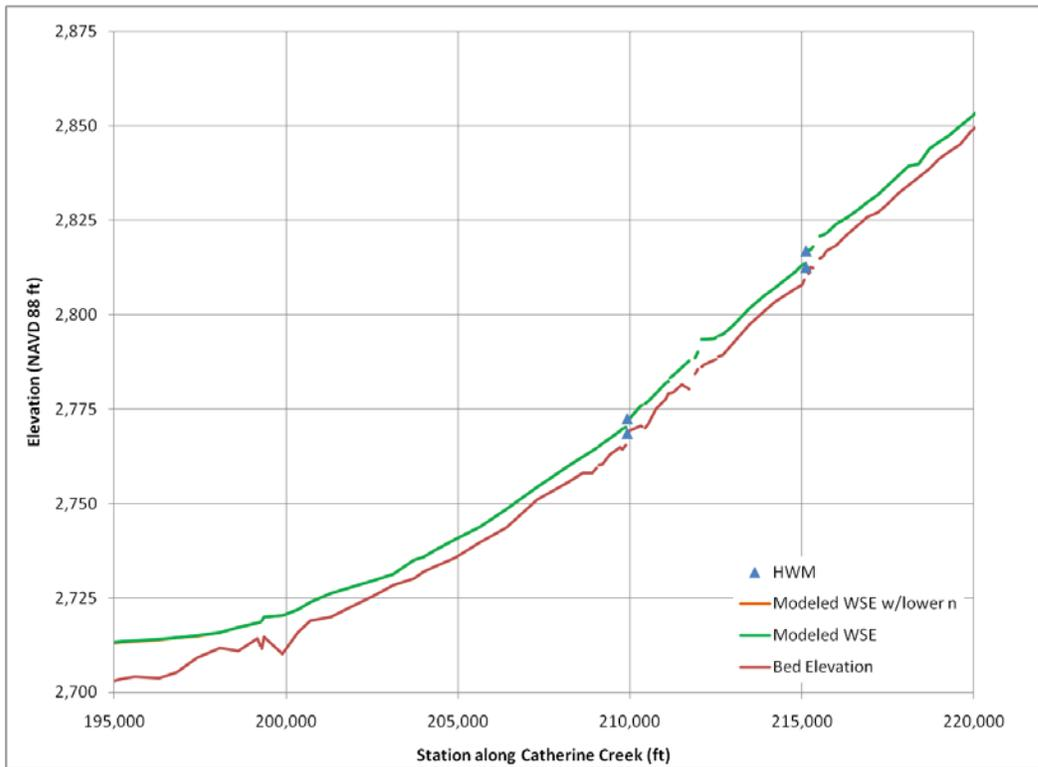
Figure 16. Modeled water surface elevations versus measured high water marks for Catherine Creek (RM 36.5 to 46.6).
