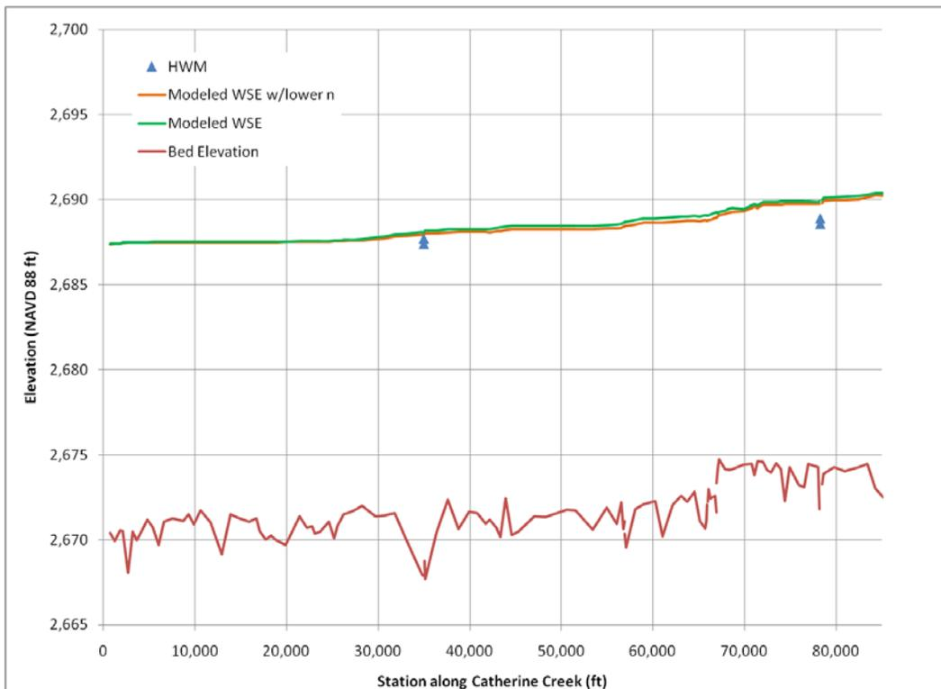
Figure 13. Modeled water surface elevations versus measured high water marks for Catherine Creek (RM 0 to 16.3).
