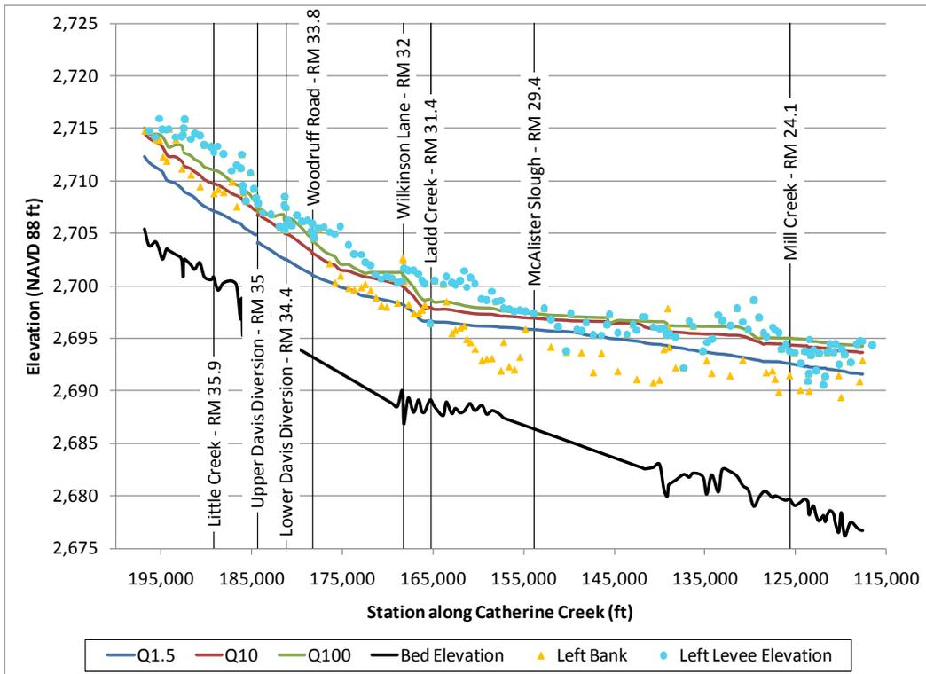
Figure 45. Reach 1 water surface profiles compared with levee and bank heights along the left bank.
