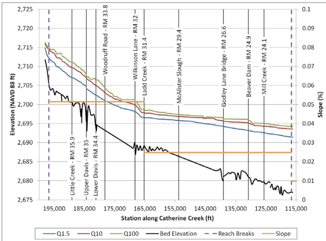
Figure 29. Computed water surface elevation for reach two on Catherine Creek.
