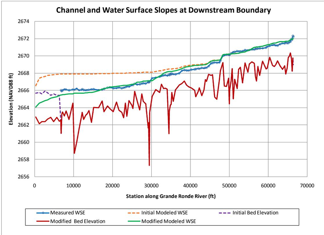
Figure 8. Illustration of changes to bed elevation at downstream end of model and resultant changes in water surface profile for a flow of 95 cfs.
