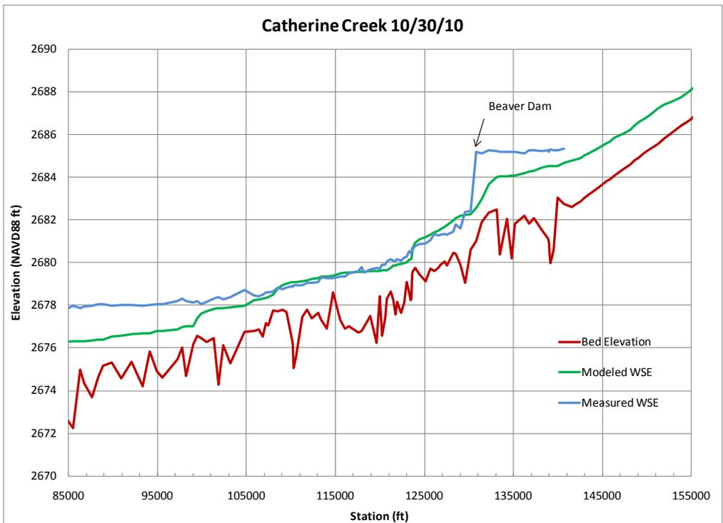
Figure 20. Measured versus modeled water surface elevations for Catherine Creek RM 16.3 to RM 29.6, measured on 10/30/2010.
