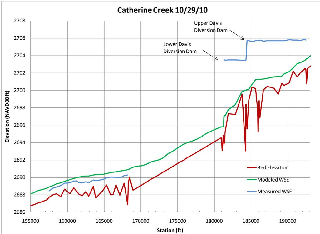
Figure 21. Measured versus modeled water surface elevations for Catherine Creek RM 29.6 to RM 36.5, measured on 10/29/2010.
