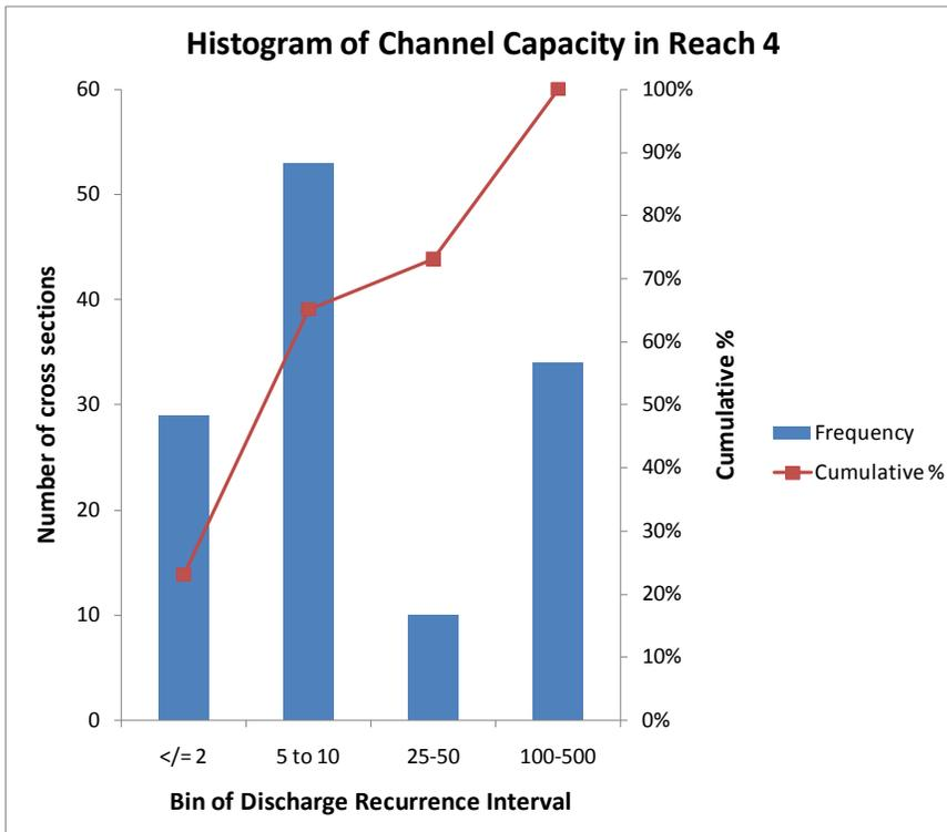
Figure 39. Distribution of channel capacity recurrence intervals for cross sections in Reach 4.
