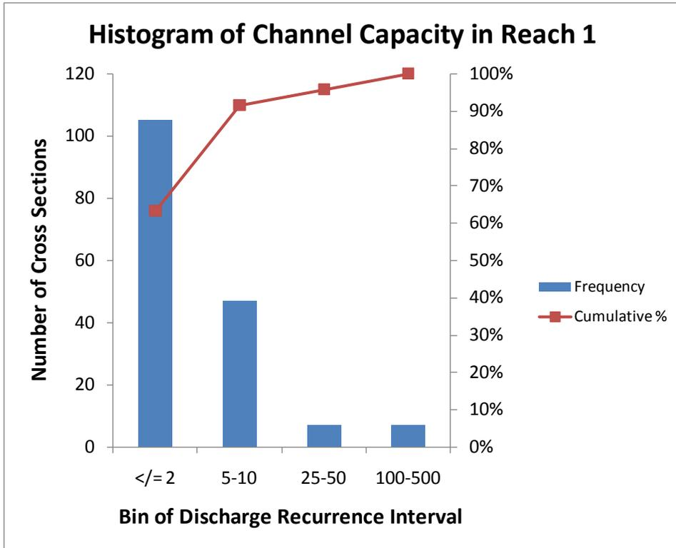
Figure 36. Distribution of channel capacity recurrence intervals for cross sections in Reach 1.
