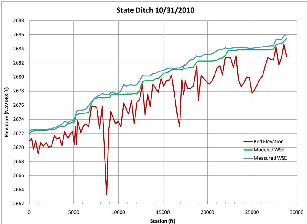
Figure 18. Measured versus modeled water surface elevations along State Ditch, measured on 10/31/2010.
