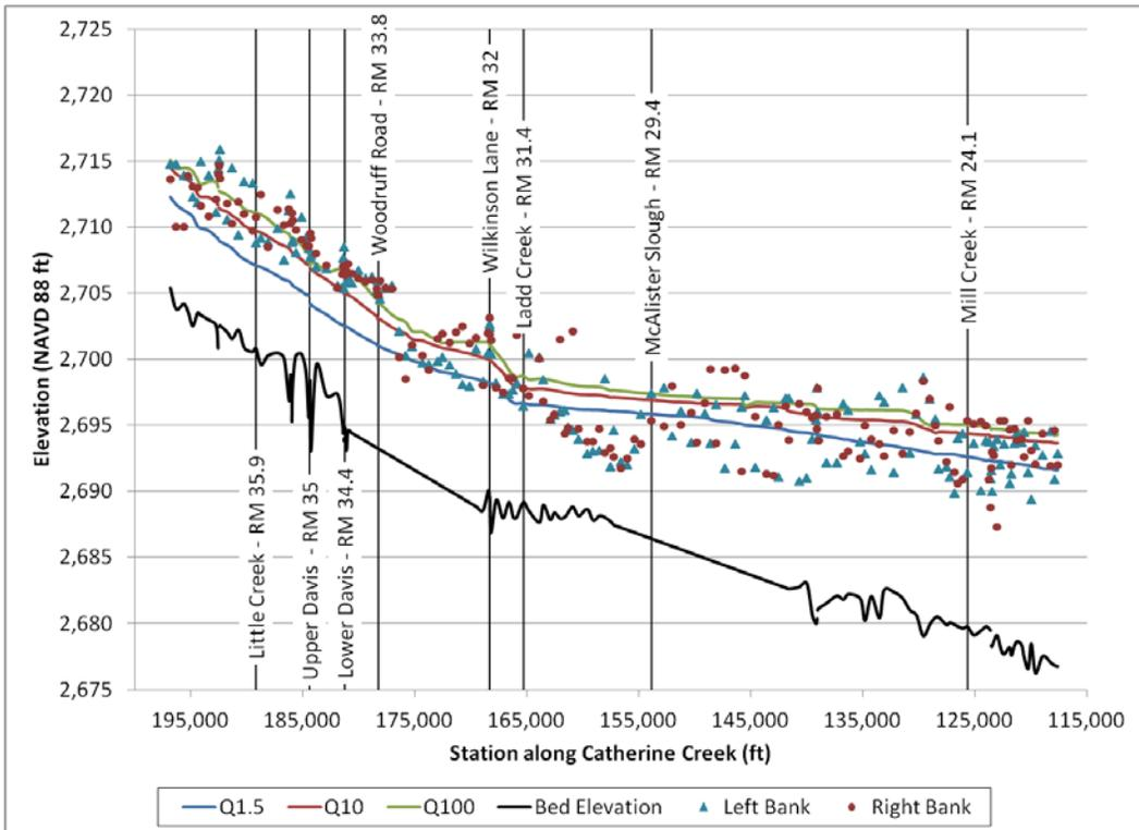
Figure 33. Comparison of bank elevations with flood discharges for Reach 2 of Catherine Creek.
