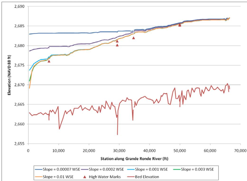
Figure 10. Comparison of different downstream boundary condition slopes for the June, 2010 discharge.
