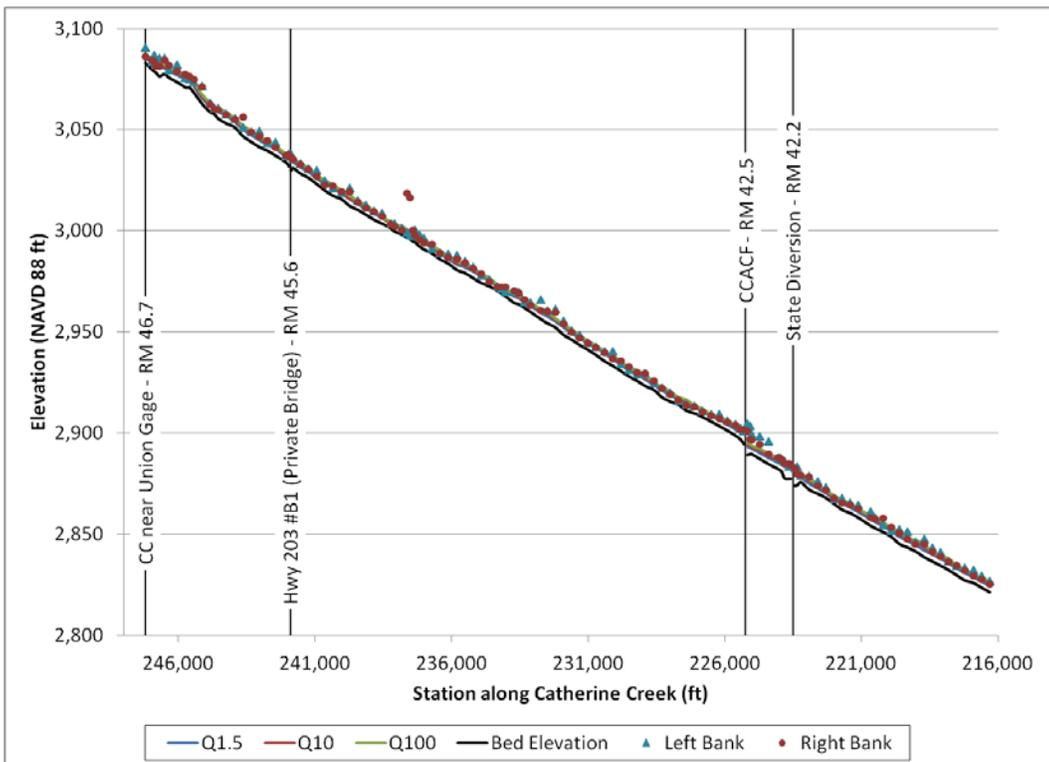
Figure 35. Comparison of bank elevations with flood discharges for Reach 4 of Catherine Creek.
