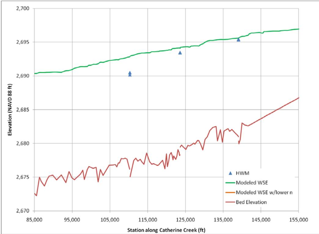
Figure 14. Modeled water surface elevations versus measured high water marks for Catherine Creek (RM 16.3 to 29.6).
