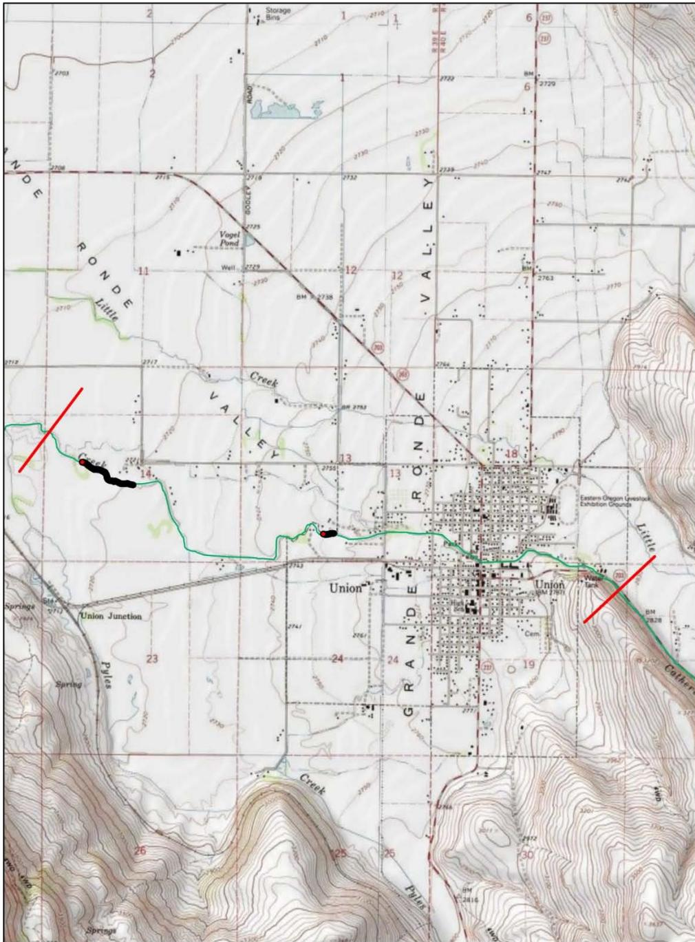
**Figure 17. Reach 3 (RM 37.2 to 40.8). Locations in reach 3 where cooler temperatures were detected during thermal profile.**
